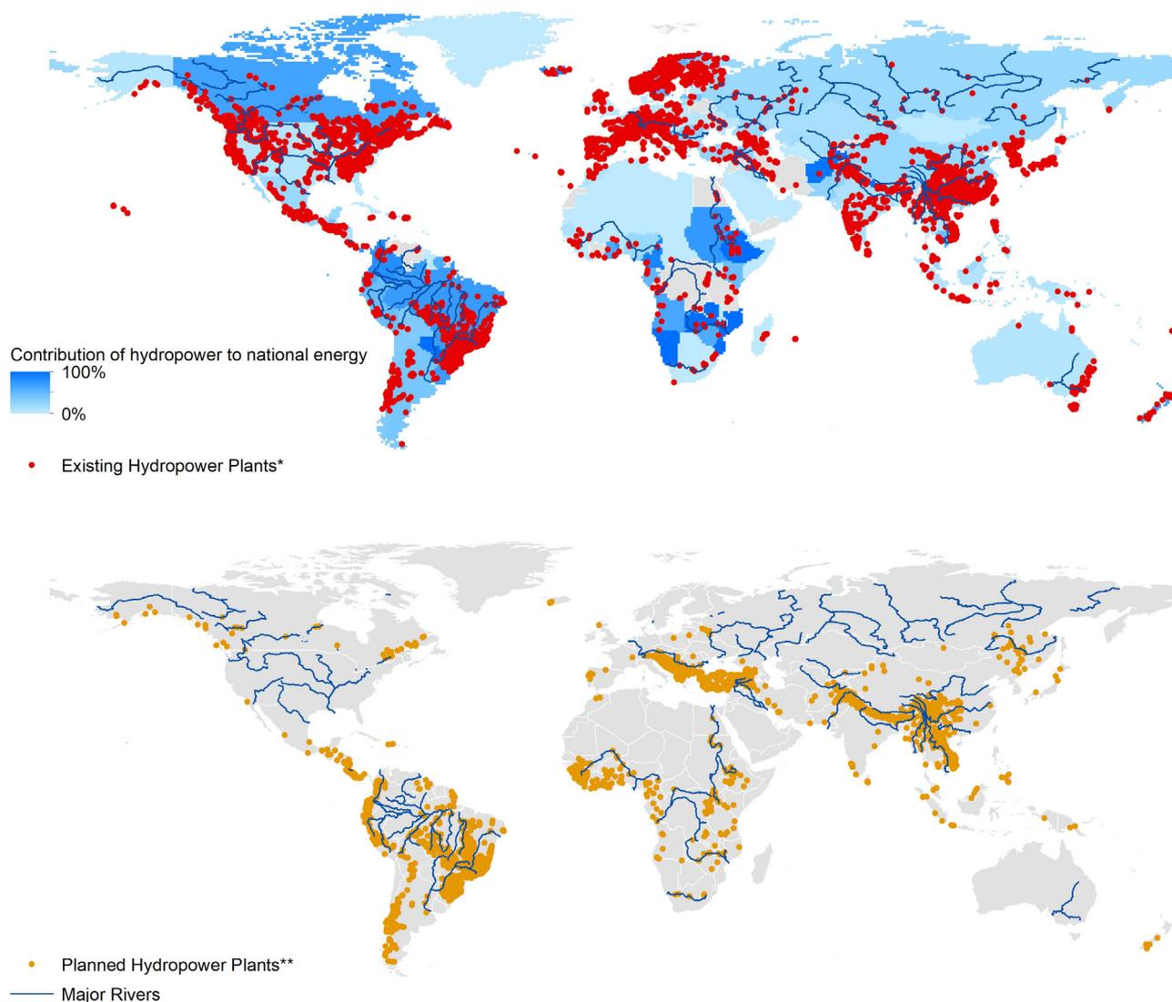
**FIGURE 1** Contribution of hydropower to the national energy mix (World Bank (2015), updated with data from IHA (2020b) for Asia and Latin America. Locations of existing hydropower plants are shown as red dots (Global Energy Observatory, 2018). Locations of hydropower plants planned for completion by 2030 are shown as orange dots (Zarfl et al., 2015)
