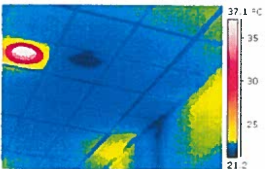
Fig. 87: A Water spot above this ceiling tile has not yet penetrated down.
