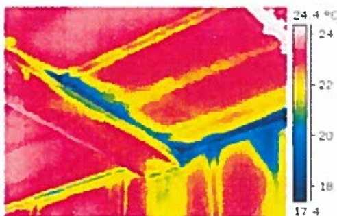
Fig. 51: Cold signatures along the junction beam and the wall-to-ceiling interface in the exercise room.
